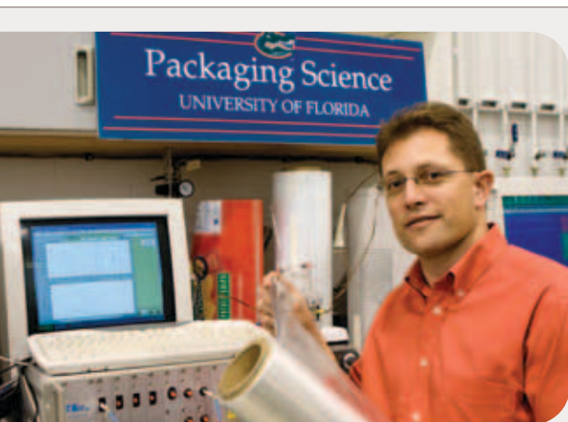
Dr. Bruce Welt, associate professor, Department of Agricultural and Biological Engineering, unwinds a multi-layer barrier film in preparation for oxygen transmission rate analysis using his newly developed unsteady state method.
